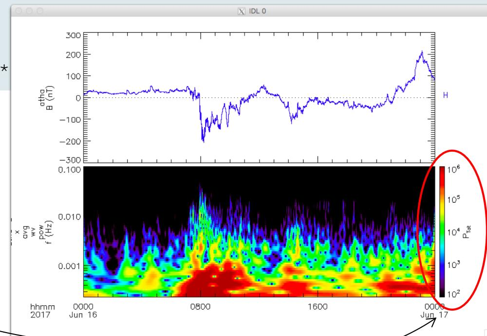
Wavelet analysis is applied to derive dynamic spectra of the data.
