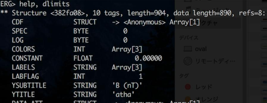
The information on the original CDF data file (CDF) and metadata, and various plot properties are extracted into a structure "dlimits".
