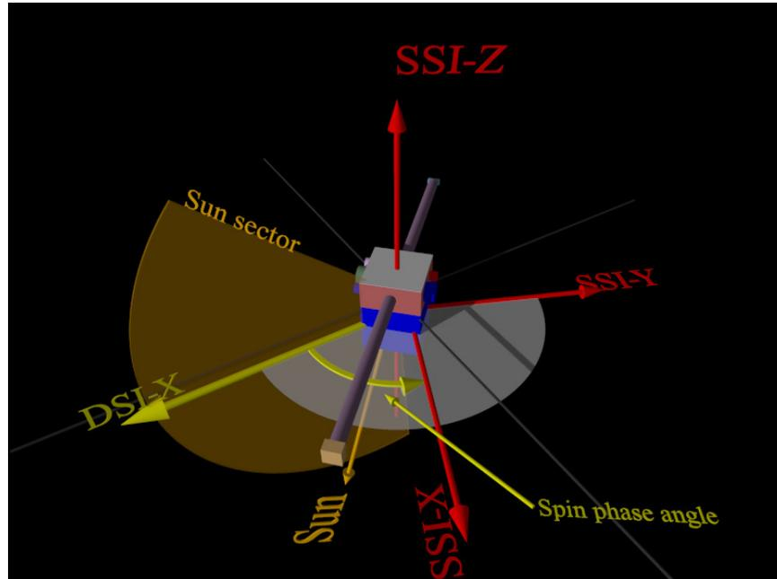
A spin period of the satellite starts when a sun pulse is detected by the SSAS-H1 (spin phase angle = 0 deg) and lasts through the next sun pulse.
