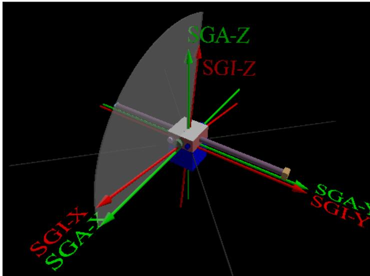
CAUTION1: This schematic shows an example in which the SGI-Z axis has an offset angle from SGA-Z about the SGA-Y axis. But SGI-Z could point in any direction, not necessarily confined in the SGA-ZX plane.
