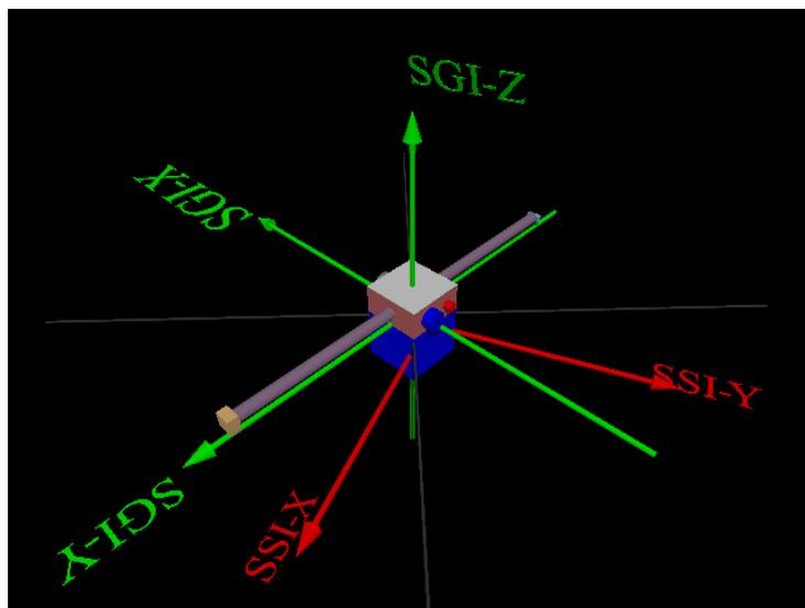
The angle between SGA-Y and the SSAS-H1 direction in the SGA-XY plane is  $\sim 21.6$  deg. Although the SGA-XY plane and the SGI-XY plane are not identical, the SSI system is close to the SGI system rotated counter-clockwise (the spin direction) by roughly  $90 + 21.6$  deg around the z-axis .
