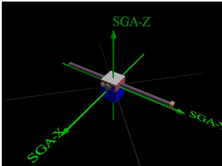
The satellite's spin direction is counter-clockwise about the z-axis, in the direction from SGA-X to SGA-Y.
